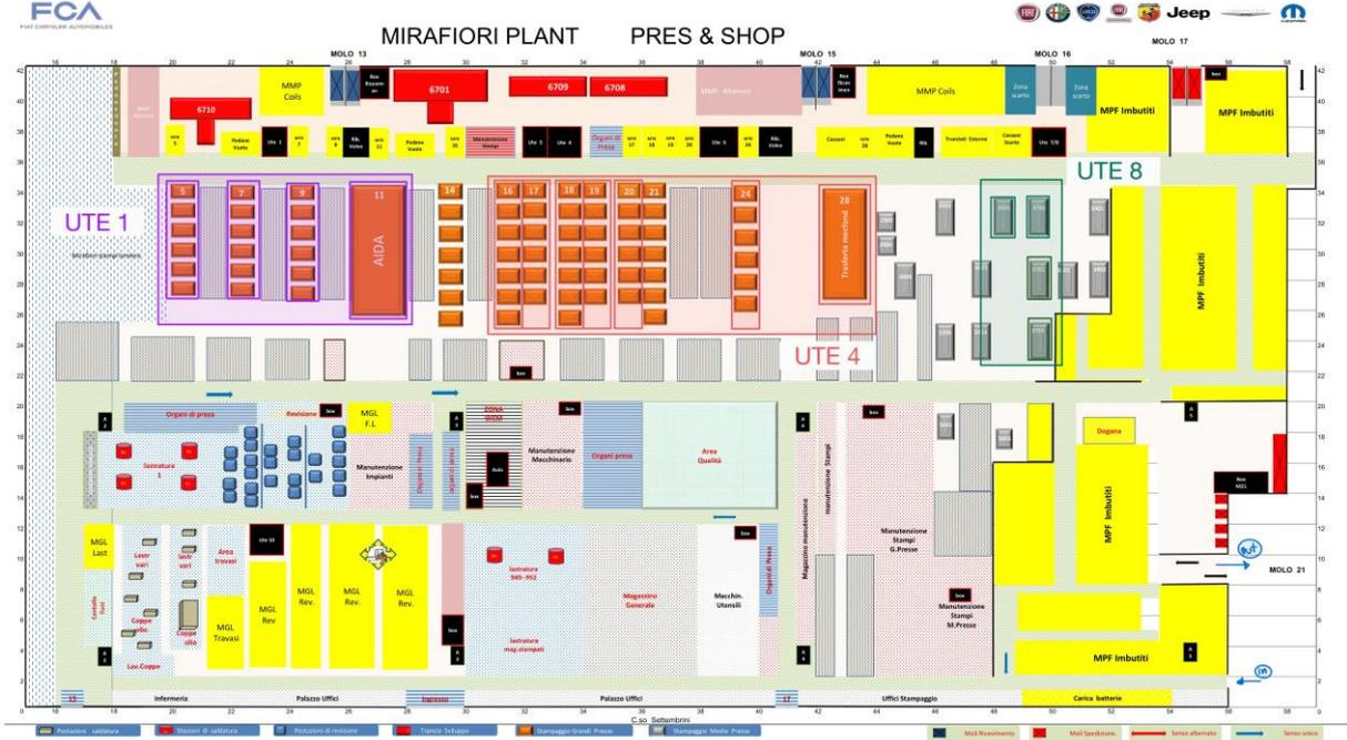
Figure 34: CRF Plant Layout
